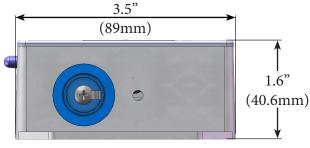
24VAC to 12VDC Mini Transformer Dimensions
